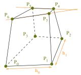
Unknowns:  $Point: P_0, P_1, \dots, P_7$ Parameters:  $Length: h_0, h_1, \dots$ Constraints:  $h_0 = distance(P_0, P_1)$   $h_1 = distance(P_0, P_2)$   $\dots$  $coplanar(P_4, P_5, P_6, P_7)$
